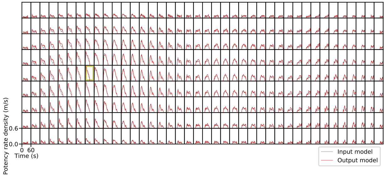
Figure 2.14: Potency rate density functions of input (our result) and output (reproduced) source models at all subfaults in the synthetic test for evaluation of our result. Gray and red traces correspond to input (our result) and output (reproduced) models, respectively. The cell outlined by yellow line represents the initially ruptured subfault.
