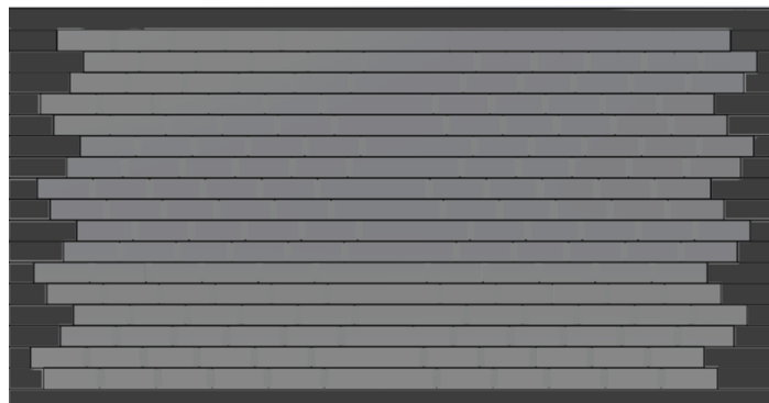
Figure 2.2.4. Lens array layer of vertical refraction decentered lens.
