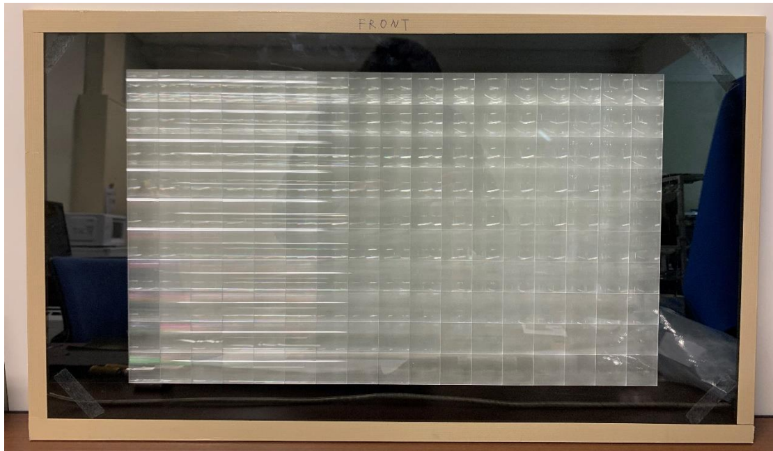
Figure 4.2.5. Image of the proposed linear Fresnel lens array with an interleaved structure.
