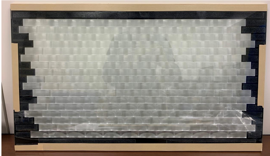
Figure 2.3.1. Lens array using decentered elemental lenses.
