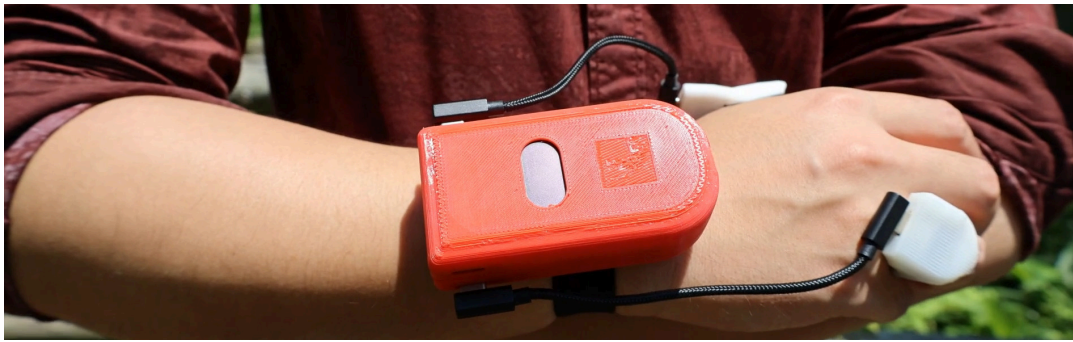
FIGURE 5.1: Custom made smart bracelet to record physiological data during the experiment.
