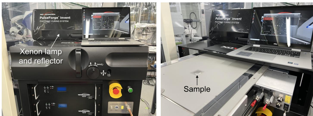
Figure 2.3. Digital images for Intense pulsed light (IPL) irradiation and the sample placement.
