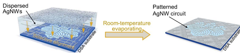
Figure 5.22. Schematic of the fabrication of AgNW TCs with arbitrary electrode designs.
