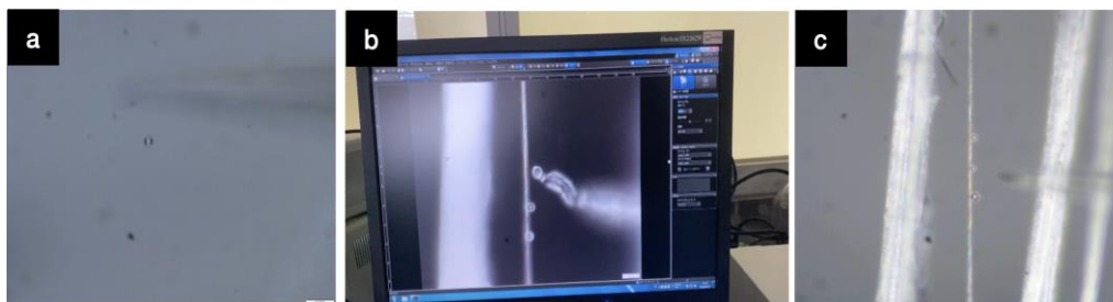
Figure 6. Pickup the microsphere a), transferring the microsphere b), and optimized the distance between the spheres (c).
