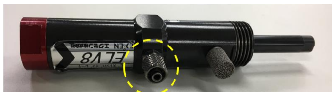
Figure 2.7.4 (a) Piston-type vibrator, (b) vibrator fixed on the attachment 2.
