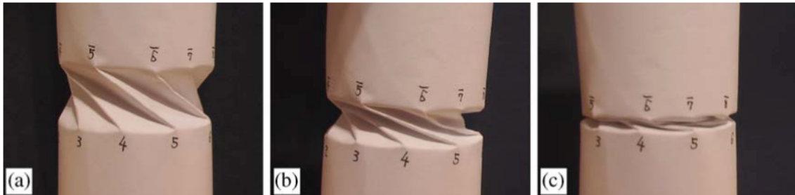
Figure 3.5: Foldable cylinder based on twist buckling of a paper roll [3].
