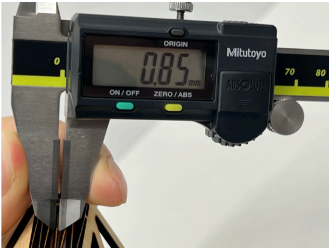
Figure 6.2: Measured local beam thickness of the structure used for the experiment in Chapter 4.
