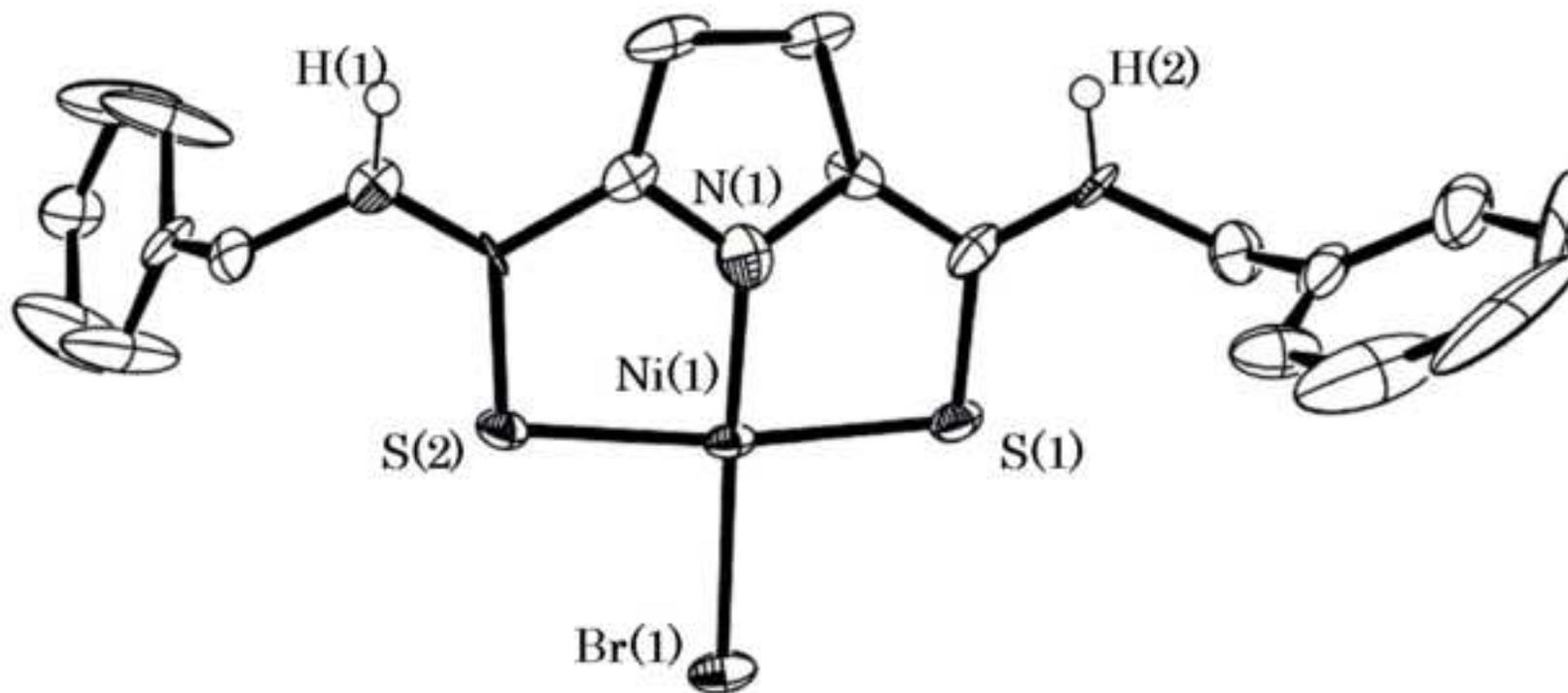
**Fig. 1.** ORTEP drawing of 2 MeCN with 50% ellipsoidal level. Hydrogen atoms except for H1 and H2 and solvated MeCN molecules are omitted for clarity.
