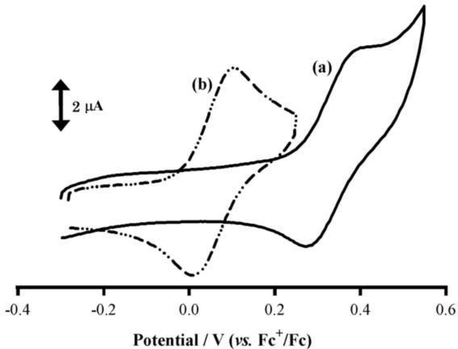
**Fig. 6.** Cyclic voltammograms of (a) **1** and (b) **4** in MeCN; 0.10 M [N(*n*-Bu)<sub>4</sub>]PF<sub>6</sub>, scan rate 50 mVs<sup>-1</sup>, glassy carbon working electrode.
