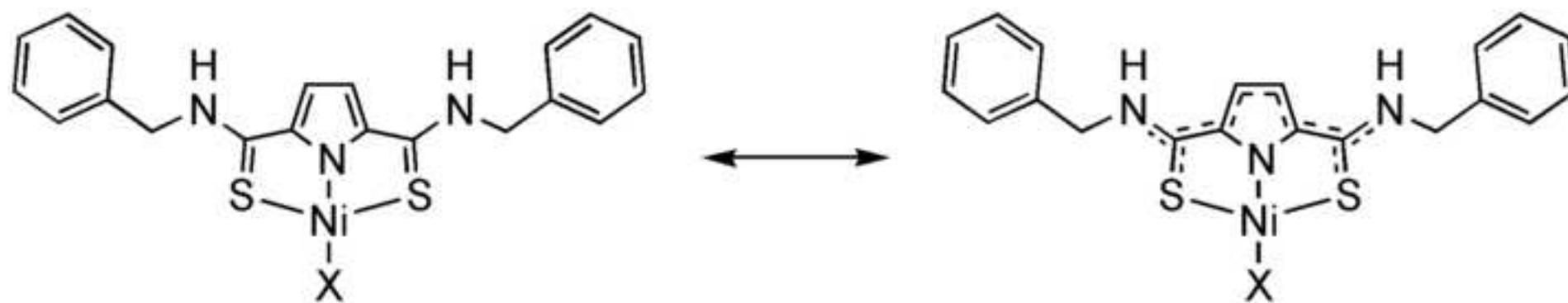
**Scheme 2.** Delocalization of electrons in the Ni(SNS) complex.
