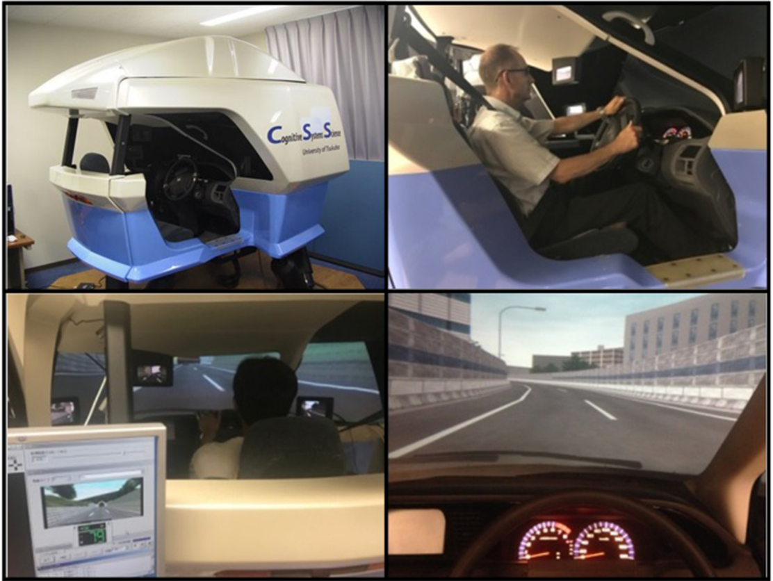
Figure 1. Honda driving simulator showing the cockpit, driver's position, and driving scene.
