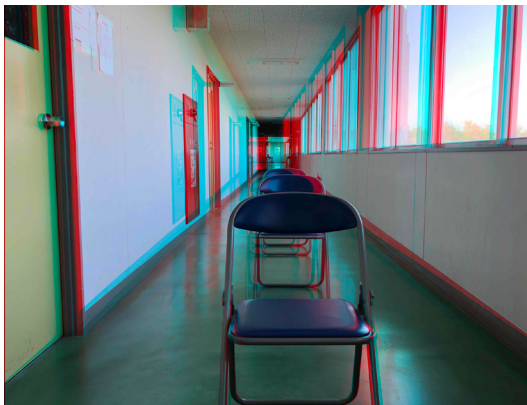
Figure 2: 3D image demonstrated by overlaid photographs of a corridor taken 6cm apart horizontally. When viewed with anaglyph glasses, the left and right eye see what the viewer would see if they were to stand in the corridor. As in real life, the brain fuses the slightly different images together to create a 3D experience.
