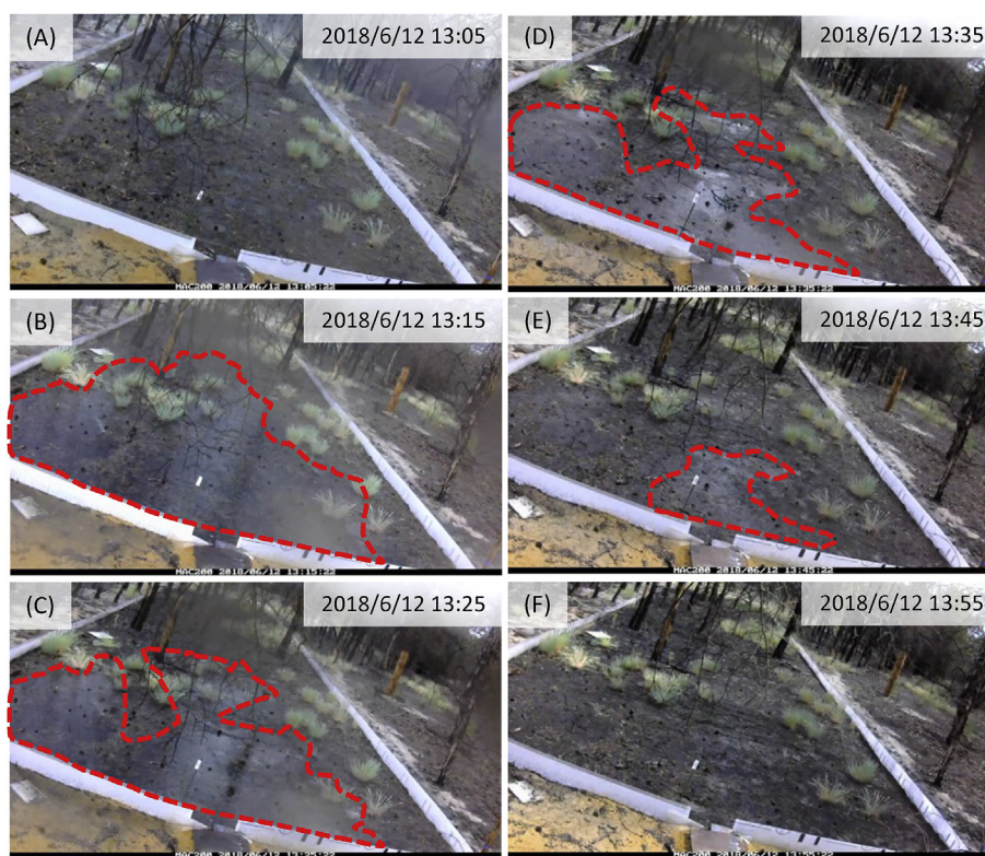
Fig. 3. Surface wash-off event on June 12, 2018 at the Red Forest (post-fire) site. The dashed line shows the saturated surface areas, which were detected with the interval camera. (For interpretation of the references to colour in this figure legend, the reader is referred to the Web version of this article.)
