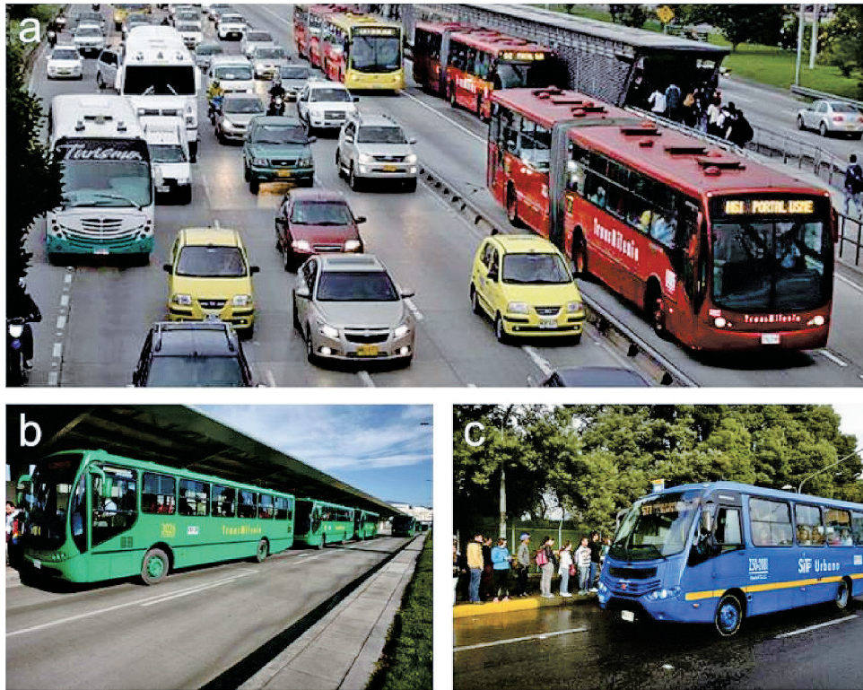
Fig. 2 Public transportation in Bogotá a: Transmilenio , b: Feeder bus, c: SITP.
