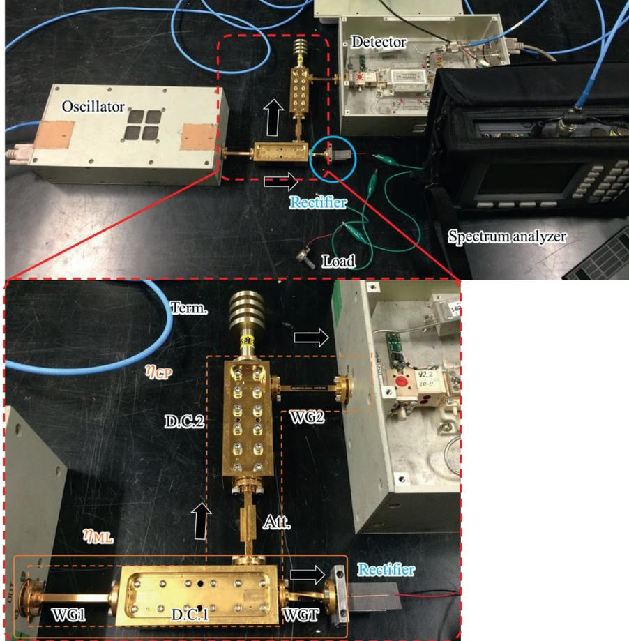
FIGURE 6: Rectifier measurement configuration. Power from the oscillator is divided at a directional coupler (D.C.1): one is input to the rectifier through the finline; the other is input to the detector. Voltage across the load is measured using the voltmeter.
