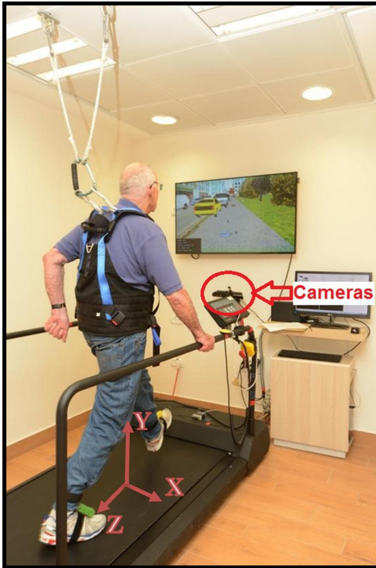
Figure 1. V-Time system. VR augmented treadmill with Kinect and HD cameras upfront for gait detection and tracking while navigating in a virtual environment. Axes orientation is as shown.
