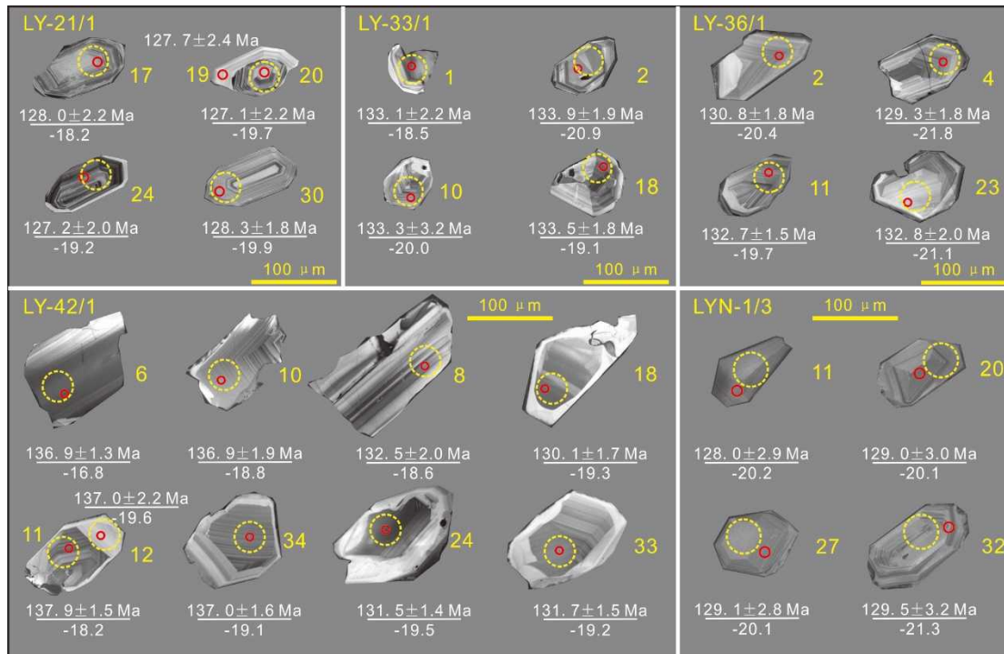
Fig. 5-2 Representative CL images of zircon grains from granitoids showing ages and \epsilon_{\text{Hf}}(t) values.
