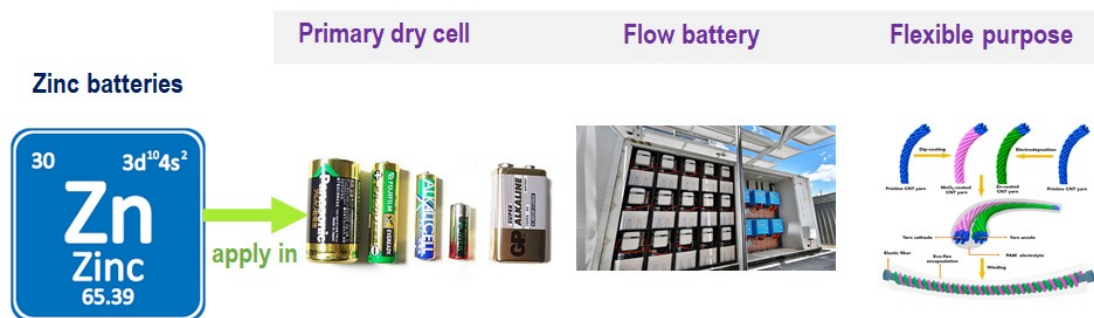
Figure 1.4 Basic property of Zn element and the application of Zn battery in primary dry cell, flow battery and flexible purpose. Pictures are harvested from https://www.electronicclinic.com/what-is-battery-types-of-battery-primary-and-secondary-cells/ (Mar.2020); https://www.sciencemag.org/news/2018/10/new-generation-flow-batteries-could-eventually-sustain-grid-powered-sun-and-wind (Oct.2018); http://www.yhcl2016.com/xinwenzixun/9.html .
