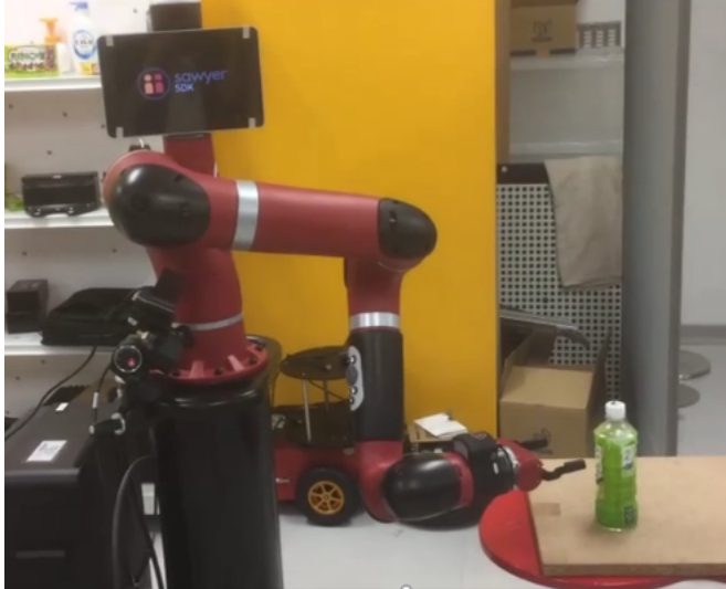
Figure 1.1: Robot manipulating a bottle - By knowing the pose of the bottle, the robot can grasp it at a desired position and orientation and place it on a shelf with the label facing the front.
