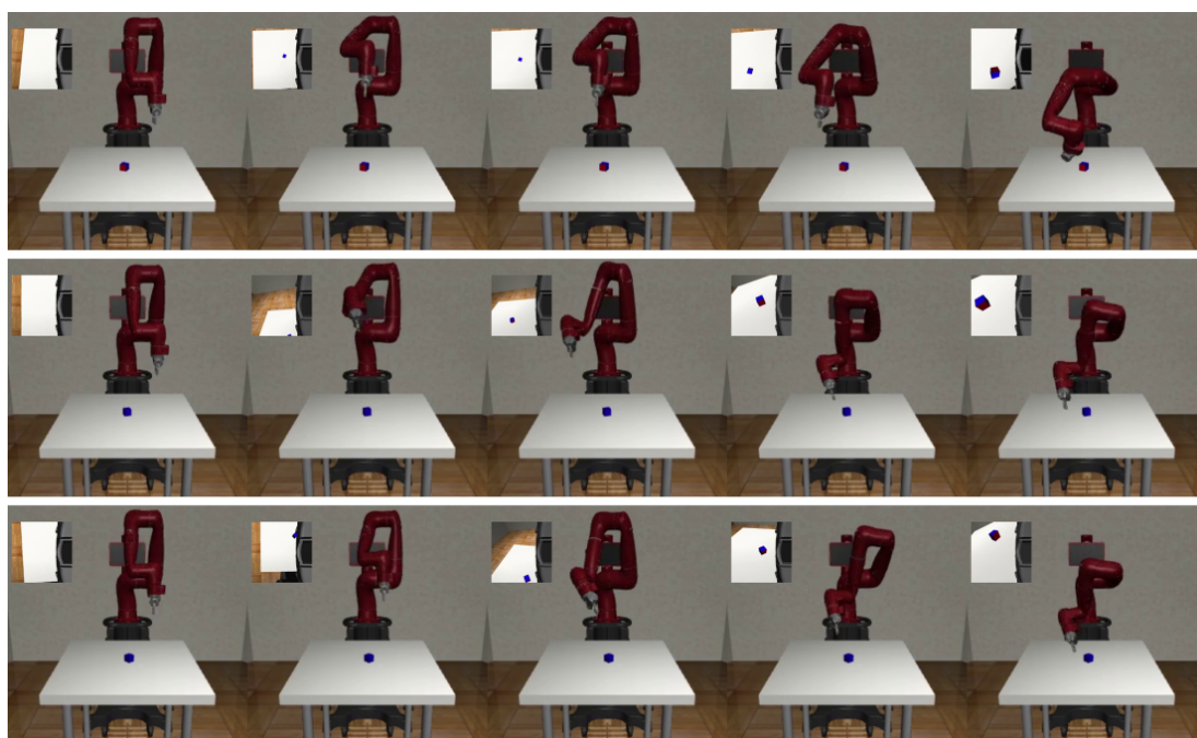
Figure 5.6: Sequences of 3 attempts at finding the best view of the cube without occlusions - The learned behaviour of the agent is to move up searching for the cube on the table and then descend facing the red side of the cube in a close view.
