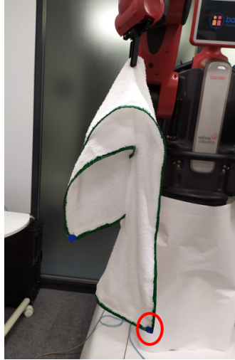
Figure 4.4: Initial position for cloth grasping - When grasping the garment from a random point, the lowest point from a frontal view corresponds to one of its corners.
