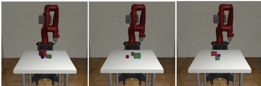
Figure 5.8: Scenario with occlusions. - As occluding objects, we add two cubes of random sizes around the target object.
