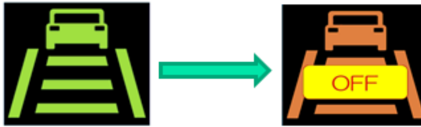
Fig. 2.3. HMI: the icon changes when automation disengages
