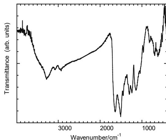
**Figure 5.** Fourier transform infrared (FT-IR) spectroscopy result of polyaniline/spider silk composite.
