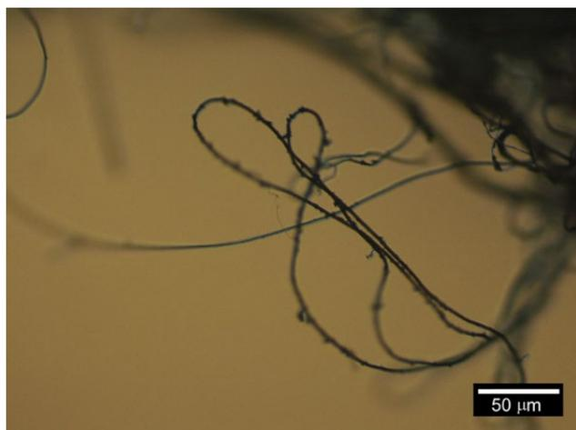
**Figure 3.** Optical microscopy image of polyaniline/spider silk composite.
