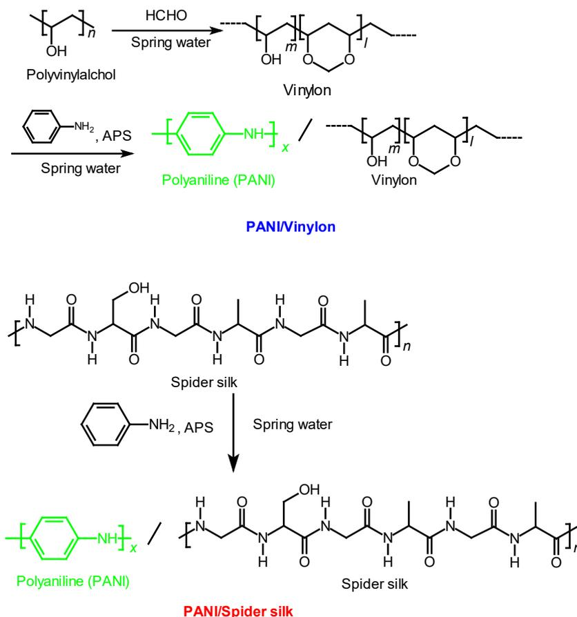
**Scheme 1.** Synthesis of PANI/vynylon and PANI/spider silk. APS = ammonium persulfate.
