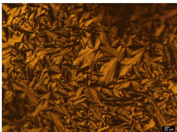
**Figure 5.** POM image of resultant polymer prepared in SmA liquid crystal.
