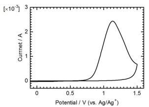
**Figure 1.** Cyclic voltammogram of P-4DMBT film in 0.1 M TBAP acetonitrile solution at scan rate of 50 mV/s.
