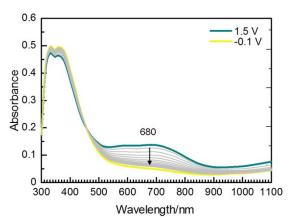
**Figure 3**. *In situ* UV-vis absorption spectra of P-4DMBT film at reduction process from 1.5 V to -0.1 V.
