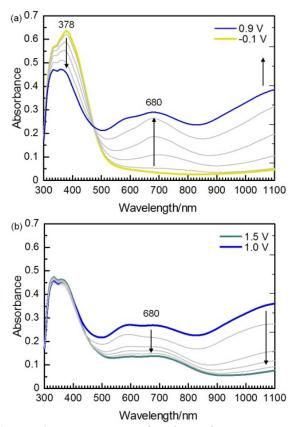
**Figure 2**. *In situ* UV-vis absorption spectra of P-4DMBT film in oxidation process. (a) -0.1 V-0.9 V, (b) 1.0 V -1.5 V.
