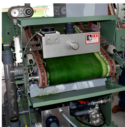
Figure 7. Drum filter equipment at Minamisoma (1.42 kW, 520 kg/h).
