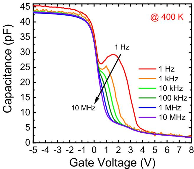
Fig. 3. Frequency dependence of  $C$ - $V$  characteristics from 1 Hz to 10 MHz at 400 K. (A colour version of this figure can be viewed online.)
