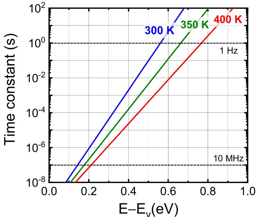
Fig. 4. Emission time constant of holes from an interface state to the valence band edge of diamond at 300, 350, and 400 K. The capture cross section was assumed to be  $1 \times 10^{-17} \text{ cm}^2$ . Two horizontal lines indicate the upper and lower frequency limits. (A colour version of this figure can be viewed online.)
