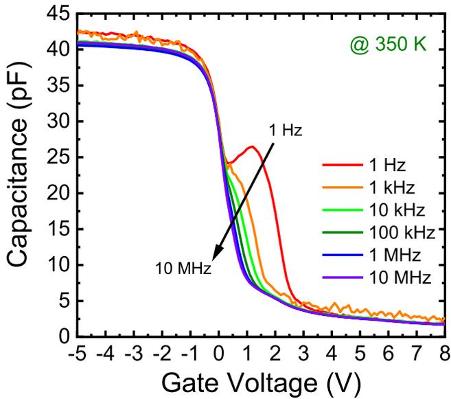
Fig. 2. Frequency dependence of  $C$ - $V$  characteristics from 1 Hz to 10 MHz at 350 K. (A colour version of this figure can be viewed online.)
