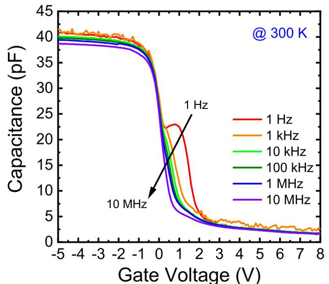
Fig. 1. Frequency dependence of  $C$ – $V$  characteristics from 1 Hz to 10 MHz at 300 K. (A colour version of this figure can be viewed online.)
