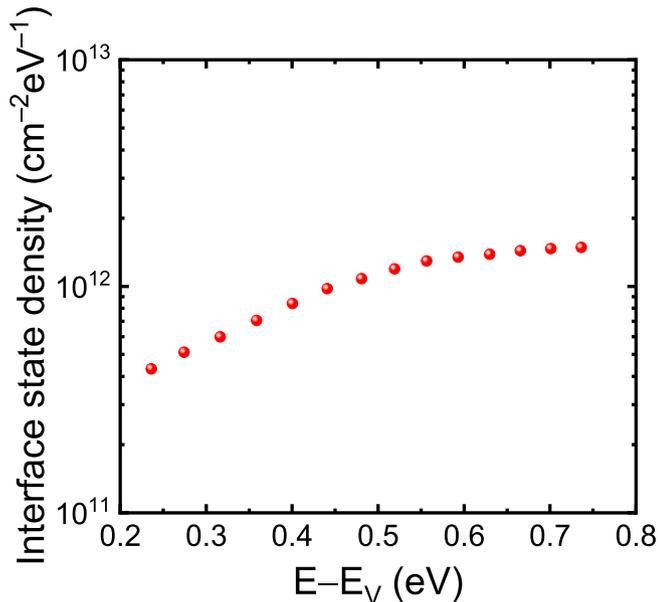
Fig. 5. Energy distribution of interface trap density ( $D_{it}$ ) for the  $\text{Al}_2\text{O}_3/\text{diamond}$  MOS structure estimated by the  $C-V$  data from 1 Hz to 10 MHz at 400 K. (A colour version of this figure can be viewed online.)
