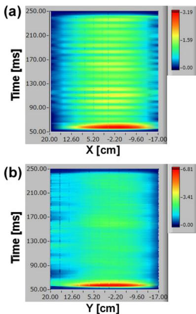
Fig. 5 Time-dependent  $H\alpha$  line emissions of the vertical array (a) and horizontal array (b).
