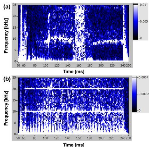
Fig. 7 Fast Fourier transform (FFT) analysis of electron line density (a) and  $H\alpha$  radiation (b).
