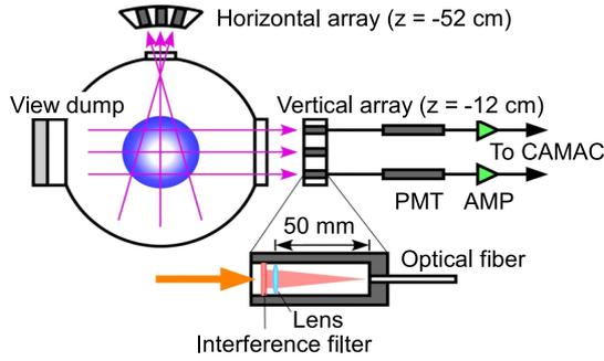
Fig. 2 Side view of the two-dimensional  $H\alpha$  line emission measurement system in the GAMMA 10/PDX central cell.
