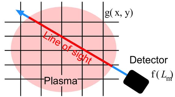
Fig. 3 Image of mesh and the line of sight.
