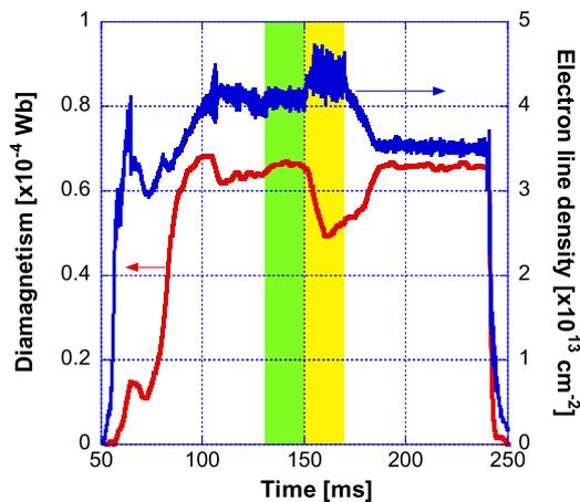
Fig. 4 Time-dependent electron line density (blue line) and diamagnetism (red line) with B-ECH (green hatched region) and P/B-ECH (yellow hatched region).
