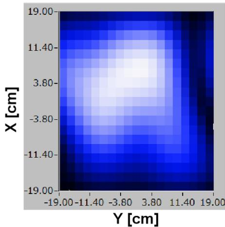
Fig. 8 Two-dimensional  $H\alpha$  fluctuation intensity obtained after the fast Fourier transform (FFT) analysis of the tomography image of emissivity at a frequency of 11 kHz at  $t = 151$  ms.
