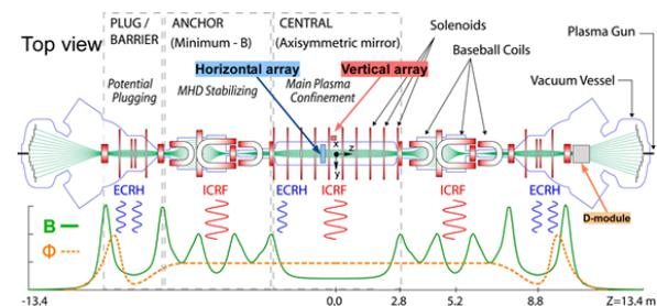
Fig. 1 Schematic view of GAMMA 10/PDX indicating the position of the vertical (red) and horizontal (blue)  $H\alpha$  array systems.
