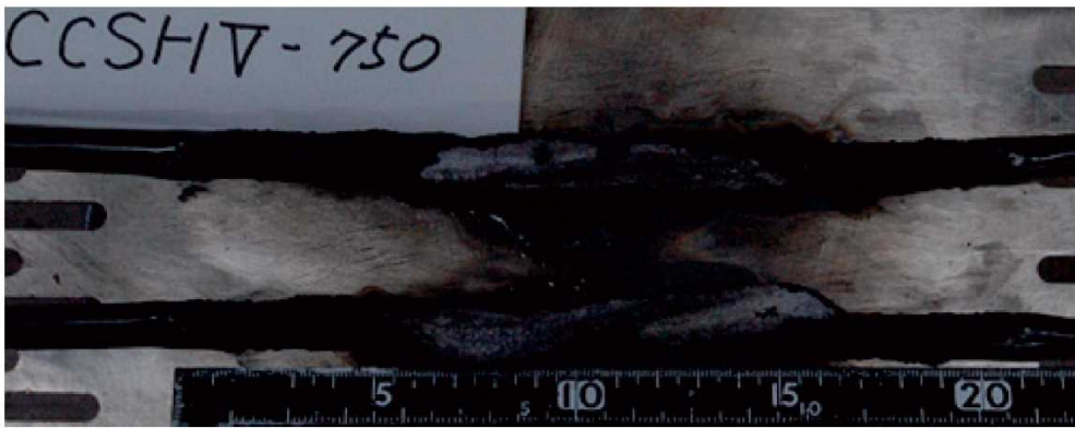
CCSHV cable temperature 490°C
