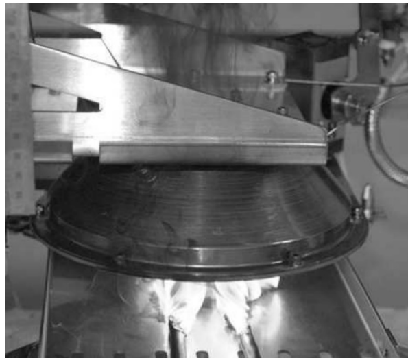
Fig. 3.4-1 View of cable heating by cone heater
