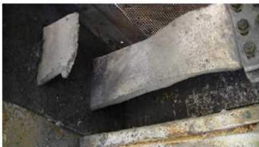
Fig. 2.5—3 SWGR Test 4 Arc 2, Cabinet 7 horizontal bus bar damage [12]
