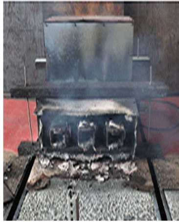
Fig. 2.5—6 Scattered granular aluminium metal at arc location in OECD/CSNI HEAF Test [3]
