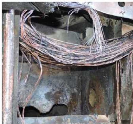
Fig. 2.5—2 SWGR Test 4 Arc 1, Cabinet 7 vertical bus bar damage [12]
