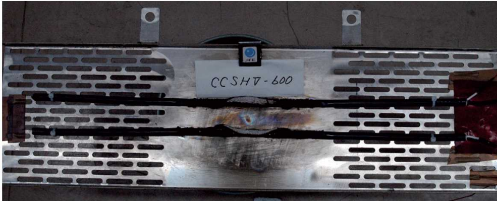
CCSHV cable temperature 340°C
