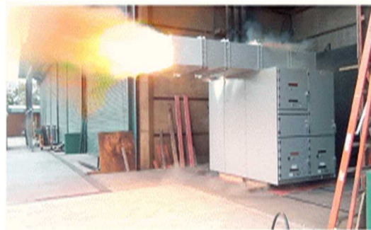
Fig. 2.6-14 Plenum exhaust for mitigating arc event (ABB Plenum Technical Guide) [22]
