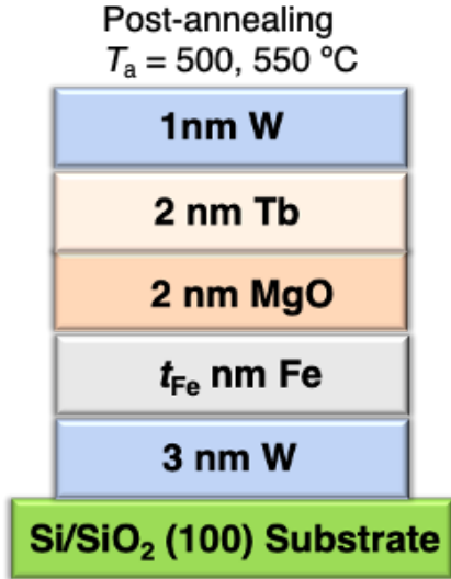
Figure 3.9 Schematic diagram of Si/SiO 2 substrate/Fe( t_{\text{Fe}} nm)/MgO/Tb/W.
