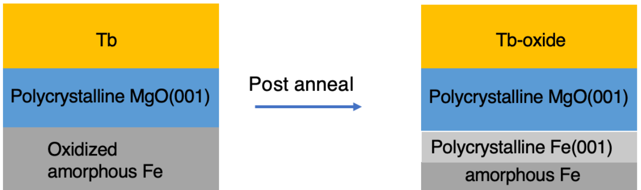
Figure 3.14 Images of as deposited and annealed samples.
