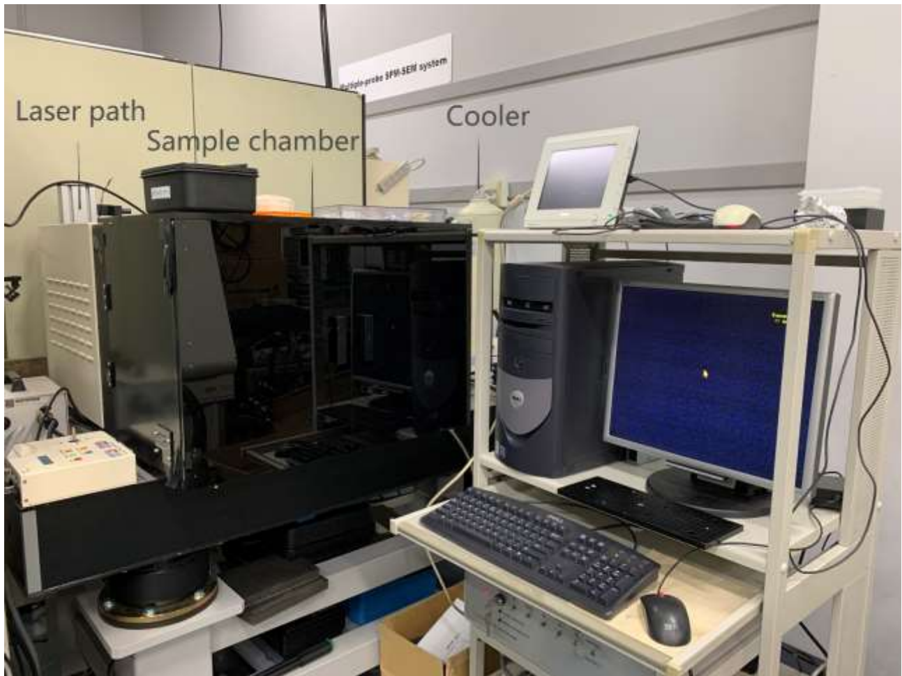
Figure A-3. Confocal HR800 micro-Raman spectrometer (Horiba Jovin Yvon), having a 100 \times objective (NA= 0.8), 532 nm diode-pumped laser (2.8mW) with the spot diameter is around 1 \mu m and a piezo-actuated XY scanner.
