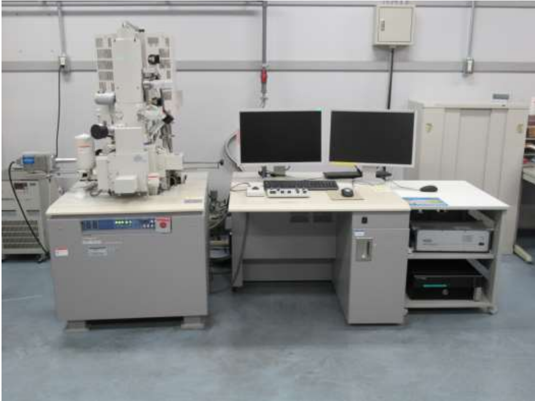
Figure A-6. Hitachi SU8000 FE-SEM with EDX (Bruker Quantax FQ5060). The accelerate voltage is 0.5 ~ 5 kV with a maximum magnification of 800k.
