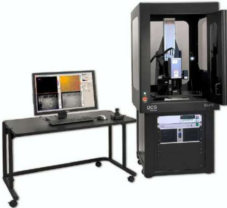
Figure A-1. Image of Enhanced Lock-in Thermal Emission (ELITE) system (DCG Systems, Inc.) for lock-in thermography measurement. The camera head contains a high-performance indium antimonide (InSb) focal plane array (FPA) detector. The FPA is cooled by a rotary stirling cooler.
