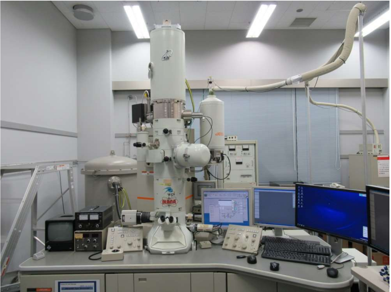
Figure A-4. JEM-2100F field emission transmission electron microscope (FE-TEM), equipped with Energy dispersive X-ray spectrometer (EDX) and electron energy loss spectrometer (EELS). The acceleration voltage is 200 kV to give an ultrahigh spatial resolution of 0.1 nm.
