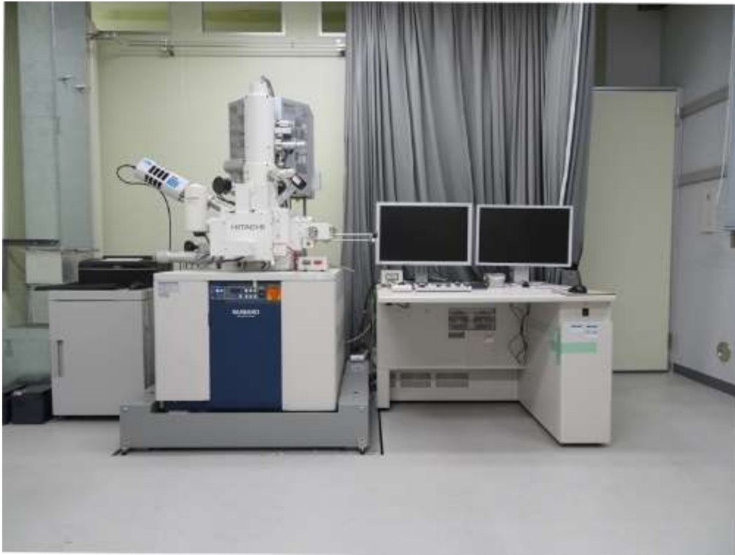
Figure A-5. Hitachi SU8230 FE-SEM with EDX. It employs a novel cold field emission gun to improve the imaging and analytical performance. The spatial resolution can be 0.8 nm (@15 kV) and 1.1 nm (@ 1kV).
