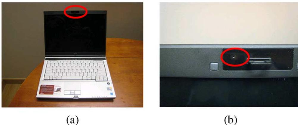
Figure 3.24: (a) Laptop with a built-in webcam and (b) close up view of the built-in camera.
