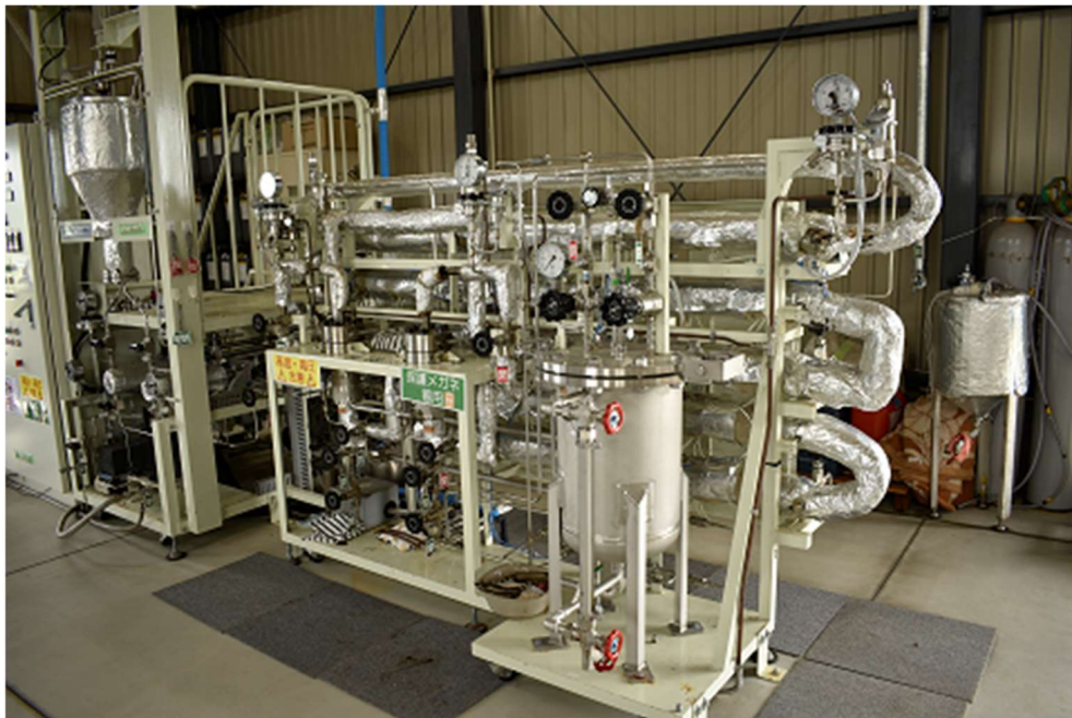
Fig. 1-10 HTL equipment at Minamisoma (10.2 kW, 21.6 kg/d)
