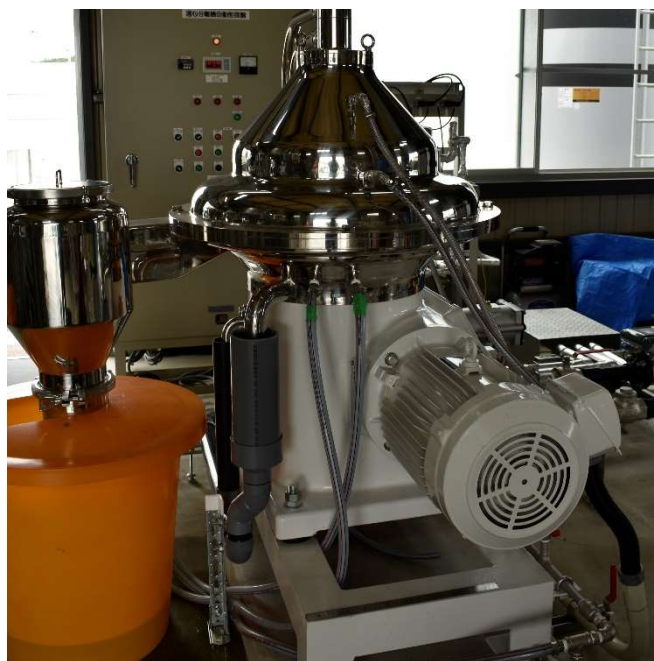
Fig. 1-6 Centrifuge equipment at Minamisoma (15 kW, 8,000 L/h)
