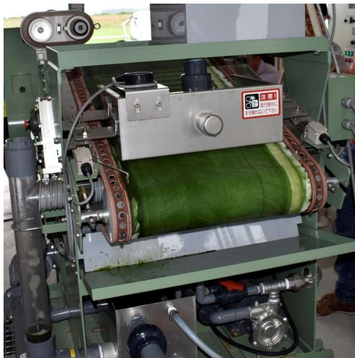
Fig. 1-8 Drum filter equipment at Minamisoma (1.42 kW, 520 kg/h)
