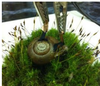
Figure 1-2-2: Implanted biofuel cell operating in a living snail [7]
