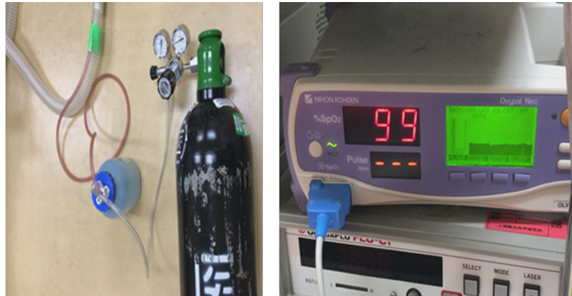
Fig. 28. Method of oxygen supplement in OE condition
