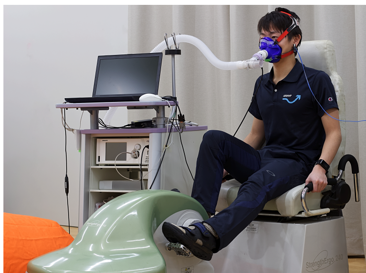
Fig. 5. Exercise under hypoxic conditions In the HY condition, participants breathed hypoxic gas, which was mixture of 13.5% O 2 and 0.03% CO 2 in N 2 (FIO 2 = 0.135), through a mask that was connected to Douglas bags. In the NO condition, participants breathed the ambient air at sea level (normoxic gas), through a mask that was connected to Douglas bags.
