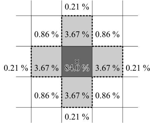
Figure 3.6: Example of the shower energy fraction in EMCal towers under assuming that a photon hit in the center of tower perpendicularly [55]. The core clusters formed by the towers contained more than 2% of total energy. In this case, surrounded five towers by dotted line is formed a core cluster.
