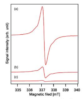
FIG. 1. The EPR spectra of H1' in the films of (a) I, (b) III, and (c) V, respectively, at 40 K. The MW frequencies are 9.45 GHz. The MW power and the amplitude of 100 kHz field modulation were 0.1 mW and 0.07 mT, respectively. The signal intensities are normalized to compare their relative intensities.
