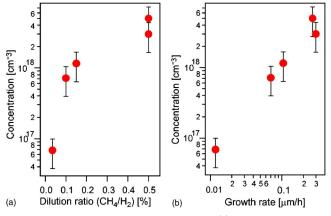
FIG. 2. The concentration of H1' with respect to (a) the  $CH_4/H_2$  ratios and (b) the growth rates.
