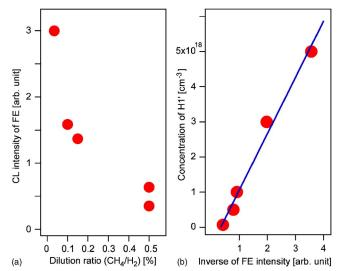
FIG. 4. The FE signal intensity with respect to  $CH_4/H_2$  ratio. (b) The concentration of H1' with respect to the FE signal intensity. The solid line in (b) is the least squares fitting curve by using Eq. (2).
