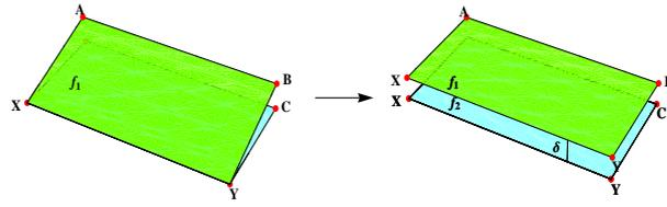
On the left, the two faces  $f_1$  and  $f_2$  share the same edge  $XY$ . On the right, the faces  $f_1$  and  $f_2$  are modeled as two plane surfaces with infinitesimally small vertical distance. The two surfaces have the same edge  $XY$  and are considered to share the same edge.
