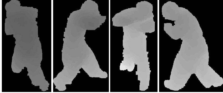
Fig. 8. Example of depth textures. Intensity of each pixel represents its depth; lighter parts are further away than darker parts.
