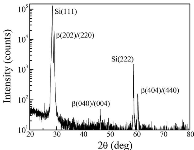
FIG. 1.  $\theta$ - $2\theta$  x-ray diffraction pattern for sample D.
