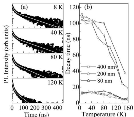
FIG. 3. Temperature dependence of (a) TR-PL decay curves for 1.54  $\mu$ m PL emission and (b) PL decay times for SFS DH.
