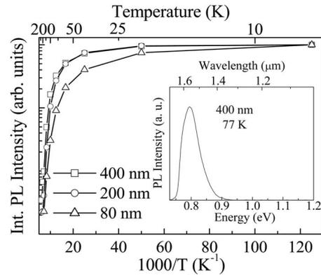
FIG. 2. Normalized temperature dependence of integrated PL intensity of 1.54  $\mu$ m emission from SFS DH with  $\beta$ -FeSi<sub>2</sub> layer thicknesses of 80, 200, and 400 nm. PL spectrum measured at 77 K was inserted.
