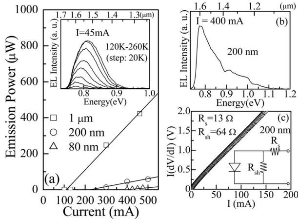
FIG. 1. (a) EL emission power with respect to injection current measured at RT for SFS DH LEDs with  $\beta$ -FeSi<sub>2</sub> layer thicknesses of 80 nm, 200 nm, and 1  $\mu$ m. Typical example of temperature dependence of EL spectra for SFS DH LED was inserted. (b) RT EL spectrum at 400 mA and (c)  $I(dV/dI)$  vs  $I$  plot for LED with a 200-nm-thick  $\beta$ -FeSi<sub>2</sub> layer.
