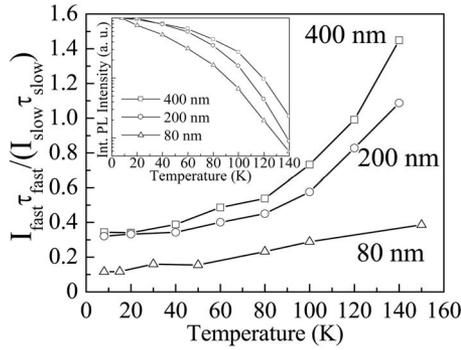
FIG. 4. Temperature dependence of PL intensity ratio ( $I_{\text{fast}}\tau_{\text{fast}}/I_{\text{slow}}\tau_{\text{slow}}$ ) for SFS DH with  $\beta$ -FeSi<sub>2</sub> layer thicknesses of 80, 200, and 400 nm. Normalized temperature dependence of integrated PL intensity of  $\beta$ -FeSi<sub>2</sub> from these samples was inserted.
