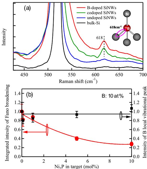
FIG. 2. (Color online) (a) Si optical phonon peaks and the B local vibrational peaks observed for B-doped SiNWs (B: 10 at%), codoped SiNWs (B: 10 at%,  $\text{Ni}_2\text{P}$ : 5 mol%), undoped SiNWs, and bulk Si. (b) Dependence of Fano broadening and the B local vibrational peak on the content of  $\text{Ni}_2\text{P}$  in the ablation targets. The micro-Raman scattering measurements were performed at an excitation power of 0.02 mW at RT.
