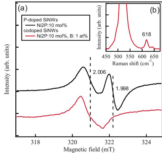
FIG. 3. (Color online) (a) ESR spectra observed for P-doped SiNWs and codoped SiNWs synthesized using  $\text{Si}_{90}(\text{Ni}_2\text{P})_{10}$  and  $\text{Si}_{98}\text{Ni}_1\text{B}_1$  targets. (b) Raman spectrum observed for the codoped SiNWs.
