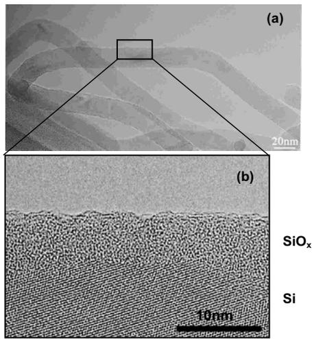
FIG. 1. Representative (a) TEM and (b) high resolution TEM images of the codoped SiNWs synthesized by laser ablation of  $\text{Si}_{95}(\text{Ni}_2\text{P})_5$  and  $\text{Si}_{99}\text{Ni}_1\text{B}_{10}$  targets.
