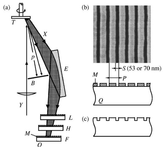
FIG. 1. (a) Experimental setup for silica nanomachining using LPSXs. (b) SEM image of a line-and-space contact mask ( $M$ ) fabricated on a silica plate ( $Q$ ). (c) Silica glass plate after irradiation with LPSXs and removal of the contact mask.
