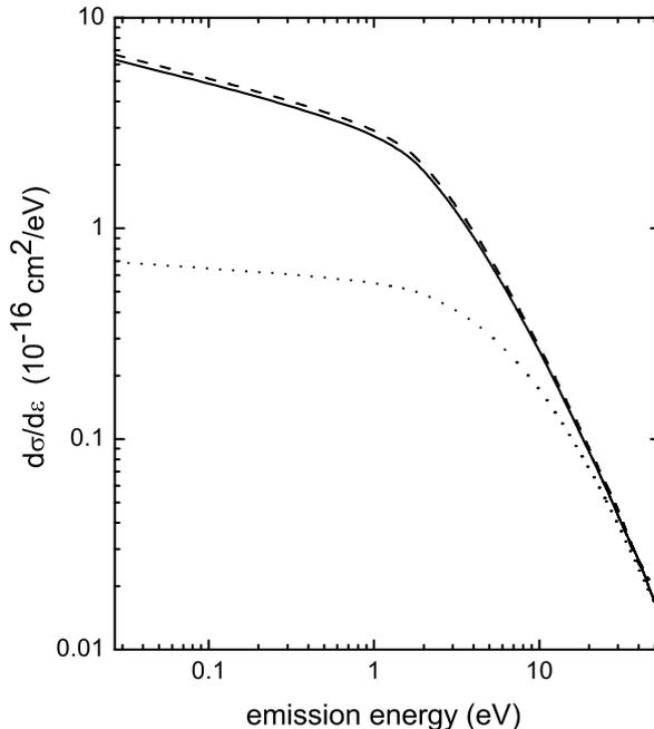
FIG. 3: Hydrogen ionization by 1 MeV/u  $C^{6+}$ . The energy spectrum of the emitted electrons,  $d\sigma/d\varepsilon_k$ . Solid and dash curves: results for  $\mathbf{F}_0 \parallel \mathbf{v}$  and  $\mathbf{F}_0 \perp \mathbf{v}$ , respectively, and zero detuning. Dot curve: results for the field-free collisions.
