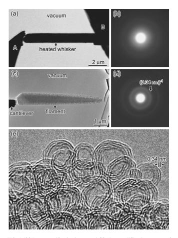
FIG. 1. (a) Low-magnification image and (b) electron diffraction pattern of a whisker prepared by heating of a  $C_{60}$  whisker. (c) Low-magnification image and (d) electron diffraction pattern of the whisker after structural change due to the impressive current. (e) High-resolution image of the surface of the whisker in (c). The whisker is composed of multilayered carbon hollow capsules of less than ten nanometers in diameter. The whisker in (c) is the filament emitting visible light.
