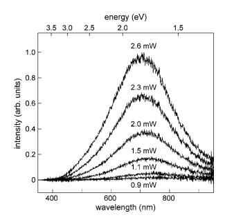
FIG. 3. Emission spectra of a whisker composed of carbon capsules at various electric powers.
