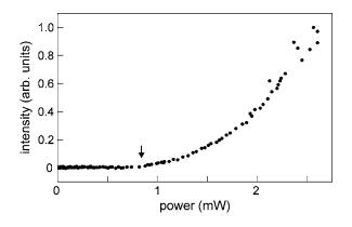
FIG. 4. Emission intensity of a whisker composed of carbon capsules as a function of the electric power.
