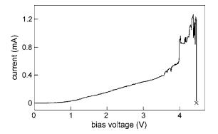
FIG. 2. Current-voltage curve of the whisker in Fig. 1(c). The abrupt increase of current at the bias voltage of 4 V indicates that the structural change occurs. Cross indicates the fracture of the contact.
