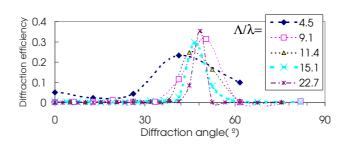
Fig. 3. (Color online) Angular distribution of the transmissive diffraction efficiency of the TE mode for case B for different  $\Lambda/\lambda$ . The aspect ratio is 1. The diffraction efficiency is connected with the auxiliary line to make it intelligible.  $\Lambda/\lambda$  is varied from 4.5 to 22.7.
