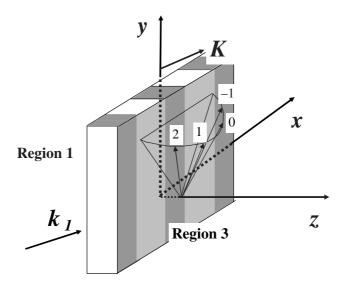
Fig. 9. Geometry of forward-diffracted wave vectors showing the conical nature of diffraction. Forward-diffracted waves (i = -1 to i = +2) are indicated by the arrow. The light travels from region 1(z < 0) to region 3(z > d).
