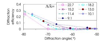
Fig. 7. (Color online) The angular distribution of the transmitted light is shown. The incidence angle is 20°, the direction of the incident light is case B, the polarization is TE,  $d/\Lambda$  is 1, and  $\Lambda/\lambda$  was varied. The angle of the peak is near 90°. The angular distribution varies greatly with  $\Lambda/\lambda$ .
