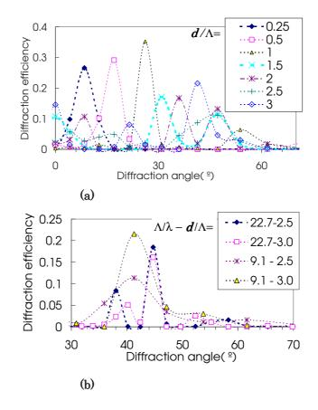
Fig. 5. (Color online) Angular distribution of the transmissive diffraction efficiency of the TE mode for different  $d/\Lambda$  for case A. The diffraction efficiency is connected with the auxiliary line to make it intelligible. (a)  $d/\Lambda$  is varied from 0.25 to 3. (b)  $d/\Lambda$  is 2.5 and 3, and  $\Lambda/\lambda$  is 9.1 and 22.7.
