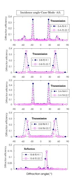
Fig. 2. (Color online) Angular distribution of the diffraction efficiency for different polarization and light directions.  $\Lambda/\lambda$  is 9.1 or 22.7. The aspect ratio is 1. Though the diffraction efficiency is discrete, it is connected with the auxiliary line to make it intelligible.
