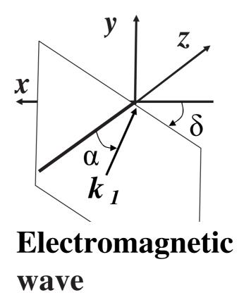
Fig. 10. A linearly polarized electromagnetic wave of wave vector  $k_1$
