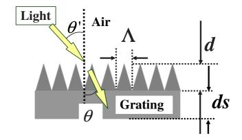
Fig. 1. (Color online) The shape of the triangular grating profile, and the definition of  $\Lambda$ , d, and ds. The fill factor is 0.5. The light direction for case A is shown. ds is assumed to be infinity. The refractive index n of the grating is 1.5.
