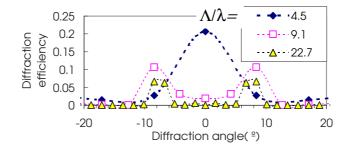
Fig. 4. (Color online) Angular distribution of the transmissive diffraction efficiency of the TE mode for case A for different  $\Lambda/\lambda$ . The aspect ratio is 2. The diffraction efficiency is connected with the auxiliary line to make it intelligible.  $\Lambda/\lambda$  is varied from 4.5 to 22.7.
