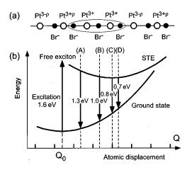
FIG. 3. (a) Schematic representation of the STE on a PtBr chain. (b) Adiabatic potential-energy curves in the configuration space.
