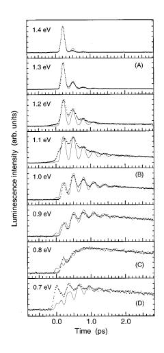
FIG. 2. Time evolution of luminescence around the onset. Dots are experimental data. Solid curves show the results of the calculation based on Eq. (4). Intensities are normalized and shown in the linear scale. The zero time delay for each photon energy has been determined by comparing the solid curves with the experimental data.
