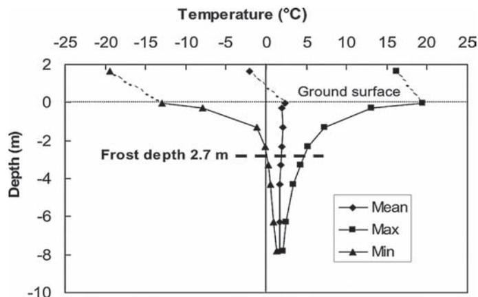
Fig. 4. Ground temperature profile in 2005–2006, indicating mean annual temperatures, maximum and minimum of mean daily temperatures and seasonal frost depth. Air temperature at 1.65 m is also shown.
