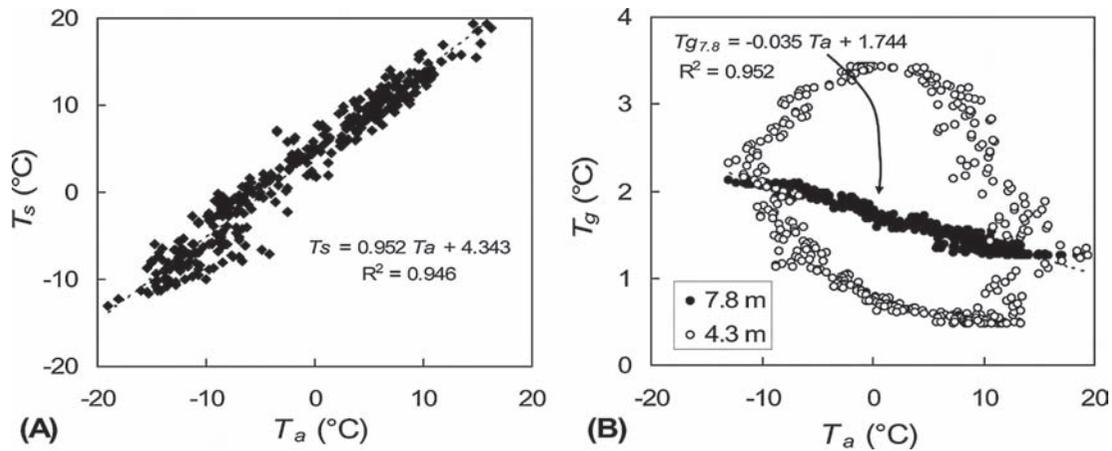
Fig. 2. Relationships between air and ground temperatures for the second year (1 August 2005 – 31 July 2006). A. Mean daily air temperatures ( $T_a$ ) versus ground surface (at 3 cm depth) temperatures ( $T_s$ ). B. Mean daily air and ground temperatures ( $T_g$ ) at 4.3 m and 7.8 m.
