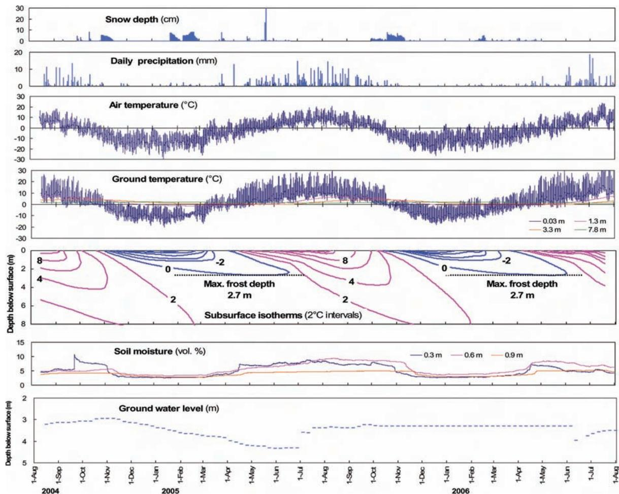
Fig. 1. Time series of environmental parameters at the Madoi observatory. Snow depth, air and ground temperature and soil moisture were monitored at 1-h intervals. The isotherms were drawn on the basis of 10-d mean ground temperatures. The groundwater level derives from weekly manual measurements.
