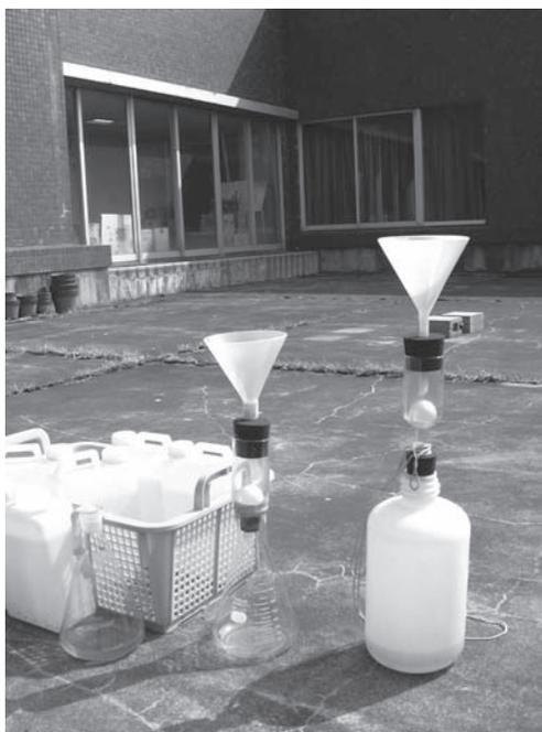
Fig.1 Photograph of the precipitation sampler with a structure which prevents the evaporation of collected precipitation. The diameter of the funnel is 12 cm.
