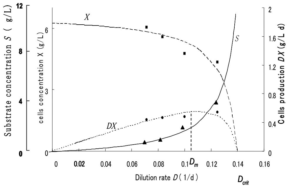
Fig.3. Dependence of cells concentration  $X$ , cells production rate  $DX$  and supply substrate concentration on continuous culture dilution rate  $D$  as simulated from Monod chemostat model. ■ cells concentration  $X$ ; ▲  $H_2/CO_2$  concentration  $S$ ; • cells production rate  $DX$ ; (—) model prediction.  $D_{crit}$  (0.14 /d).
