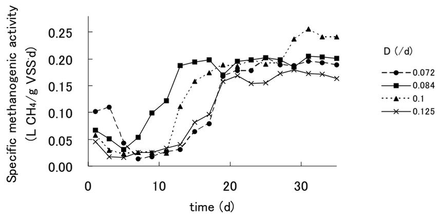
Fig.2. Time course of the Specific Methanogenic Activity (SMA) during the experiment time (days) at different dilution rate; the SMA was obtained from the relation between the bacteria growth rate and the methane production rate at mesophilic temperature ( $37 \pm 2^\circ\text{C}$ ).
