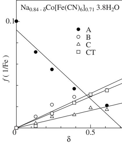
FIG. 8. Oscillator strength  $f$  of thin films of  $\text{Na}_{0.84-\delta}\text{Co}[\text{Fe}(\text{CN})_6]_{0.71} \cdot 3.8\text{H}_2\text{O}$  at 300 K. The straight lines are the least-squares-fitted results.
