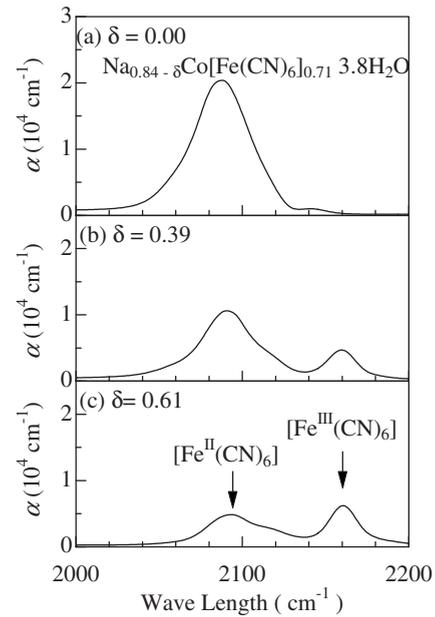
FIG. 2. Infrared absorption spectra of thin films of  $\text{Na}_{0.84-\delta}\text{Co}[\text{Fe}(\text{CN})_6]_{0.71} \cdot 3.8\text{H}_2\text{O}$  measured at 300 K: (a)  $\delta=0.00$ , (b)  $\delta=0.39$ , and (c)  $\delta=0.61$ . The higher- and lower-lying bands are ascribed to the CN stretching vibration of  $[\text{Fe}^{\text{II}}(\text{CN})_6]$  and  $[\text{Fe}^{\text{III}}(\text{CN})_6]$ , respectively.
