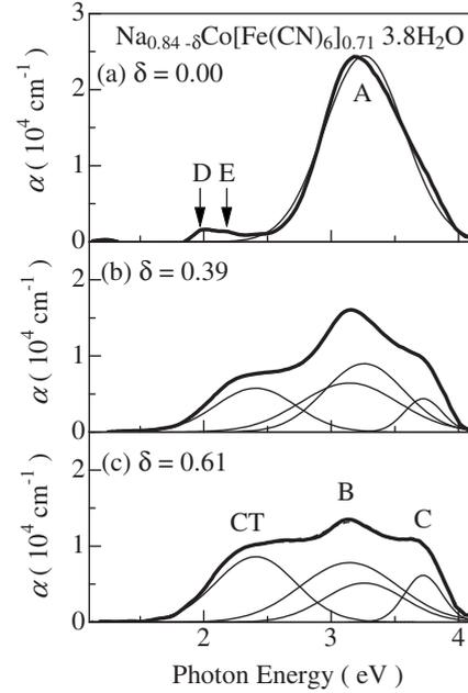
FIG. 7. Absorption spectra of thin films of  $\text{Na}_{0.84-\delta}\text{Co}[\text{Fe}(\text{CN})_6]_{0.71} \cdot 3.8\text{H}_2\text{O}$  measured at 300 K: (a)  $\delta=0.00$ , (b)  $\delta=0.39$ , and (c)  $\delta=0.61$ . The thin curves represent the least-squares-fitting with the four Gauss-type absorption bands (the A, B, C, and CT bands). D and E bands can be ascribed to the intra-atomic  $d-d$  transition of  $\text{Co}^{2+}$  (see text).
