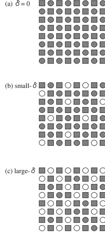
FIG. 9. Schematic illustrations of hole-doped  $\text{Co}^{2+}\text{-Fe}^{2+}$  system: (a)  $\delta=0$ , (b) small  $\delta$ , and (c) large  $\delta$ . Circles and squares represent the Fe and Co site, respectively. White color indicates the hole site ( $\text{Fe}^{3+}$ ).
