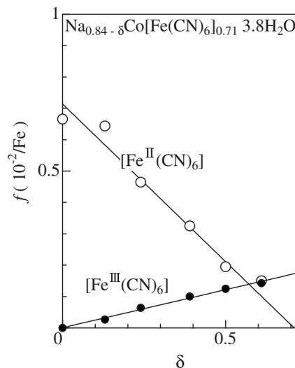
FIG. 3. Oscillator strength  $f$  of the CN stretching vibration of  $[\text{Fe}^{\text{II}}(\text{CN})_6]$  and  $[\text{Fe}^{\text{III}}(\text{CN})_6]$  at 300 K. The straight lines are the least-squares-fitted results.
