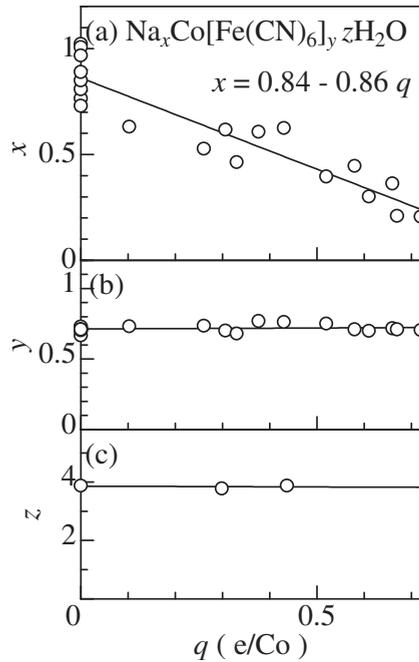
FIG. 1. Chemical composition of  $\text{Na}_x\text{Co}[\text{Fe}(\text{CN})_6]_y \cdot z\text{H}_2\text{O}$  films against the total charge  $q$  used in the oxidation process: (a)  $x$ , (b)  $y$ , and (c)  $z$ . The chemical composition was determined by the elemental analysis by the ICP method and the CNH organic elementary analyzer.
