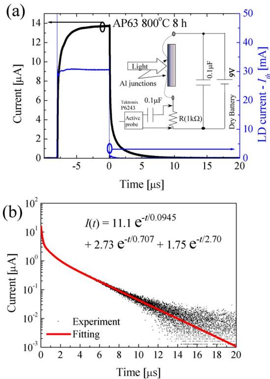
FIG. 3. (Color online) (a). Decay curve of photoconductivity (thick line) and LD drive current (thin line) with time measured at RT using a 1.31  $\mu\text{m}$  light pulse. The measurement circuit was inserted. (b) Semilogarithmic plot of photoconductivity with time and fitting using three decay times.
