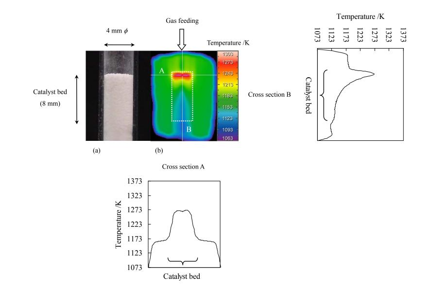
Fig. 1. Picture of catalyst granules in the quartz glass tube (a) before reaction at room temperature and (b) one example of thermographical image during the oxidative steam reforming of methane.
