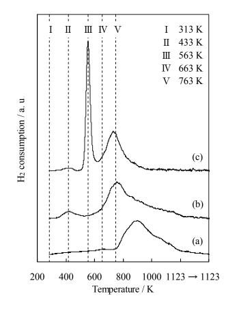
Fig. 3. Temperature-programmed reduction profiles of fresh catalysts.
