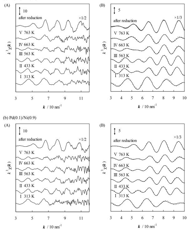
Fig. 5. Results of Pd *K*-edge XAFS analysis of Pd(0.1)+Ni(0.9) (a) and Pd(0.1)/Ni(0.9) (b) catalysts: (A)  $k^3$ -weighted oscillations; (B) Inversely Fourier filtered data (solid line) and calculated data (dotted line) based on the curve fitting results listed in Tables 3 and 4.
