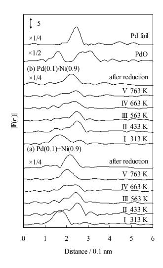
Fig. 4. Results of Fourier transform of Pd *K*-edge XAFS oscillation of (a) Pd(0.1)+Ni(0.9) and (b) Pd(0.1)/Ni(0.9) during the H<sub>2</sub> reduction and after H<sub>2</sub> reduction. The results of Ni foil, Pd foil, and PdO are also shown as a reference.
