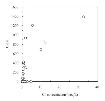
Fig. 10 Cl<sup>-</sup> concentration versus Cl/Br ratio of the groundwater.
