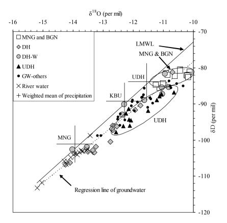
Fig. 4  $\delta^{18}$ O versus  $\delta$ D in the groundwater and annual volume weighted mean precipitation. DH-W denotes the western region of DH. GW-others denotes the groundwater at KBU, DGH, and JGH. River water denotes the data of the main stream of the Kherlen River.
