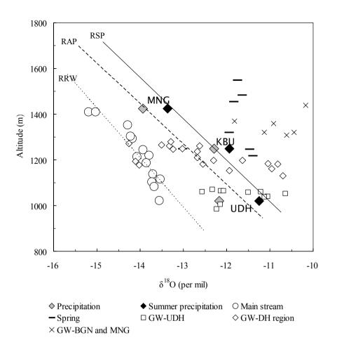
Fig. 12 The altitude versus  $\delta^{18}$ O of the river water, groundwater, spring water and annual / summer volume weighted mean precipitation. GW denotes the groundwater, and 'GW-DH' denotes the DH and DH-W regions combined. RRW: regression line of the river water, RAP: regression line of the annual volume weighted mean precipitation, RSP: regression line of the volume weighted mean precipitation in the summer season (April – October).
