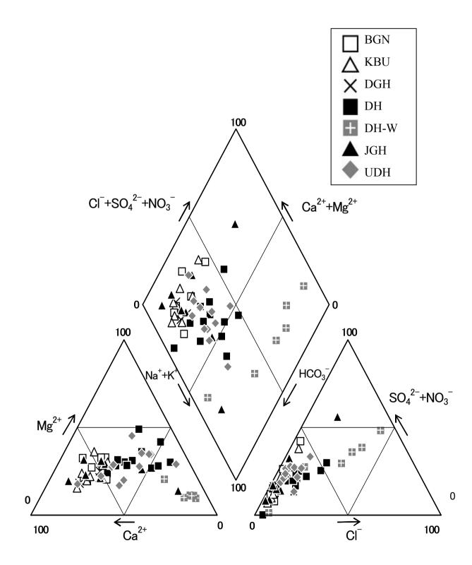
Fig. 8 Trilinear diagram of the groundwater samples.
