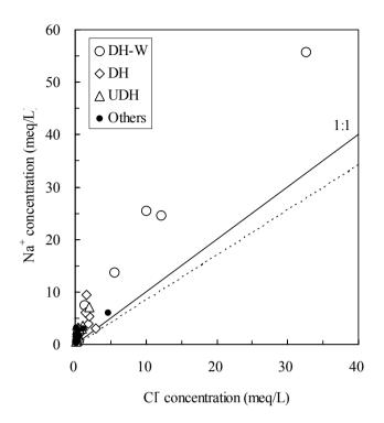
Fig. 9 The Cl<sup>-</sup> versus Na<sup>+</sup> concentration of the groundwater. The dotted line shows the ocean water line. 'Others' denotes all data except for DH-W, DH and UDH.
